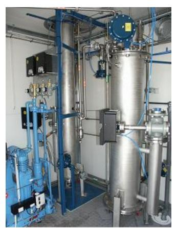
**Figure 7.** Biogas upgrading unit (water scrubber) at Plönninge biogas plant, Sweden. (Source: Courtsey: BioRega, Sweden; Peter Karlsson, Biogas Öst seminarium 2011-04-01)
