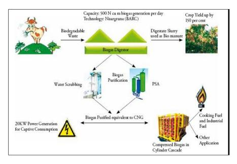
**Figure 15.** Schematic diagram of biogas upgrading and bottling plant at Nasik, Maharashtra (Source: Prof. V. K. Vijay, IIT Delhi, India)
