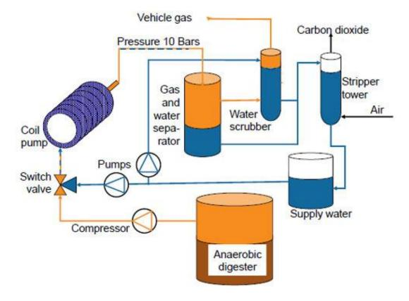
Figure 3. BioSling process flow diagram (Courtesy: Artic Nova, Sweden).
