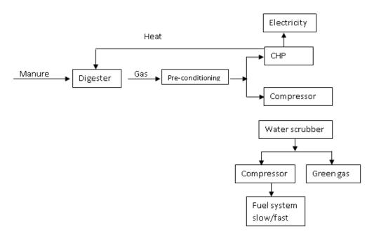
**Figure 2.** Process scheme biogas utilisation at Zalaergerzeg WWTP, Hungary (Courtesy, DMT Environmental Technology, The Netherlands)
