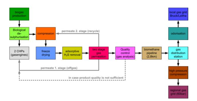
**Figure 6.** Process integration of the biogas upgrading plant Bruck an der Leitha (Source: Virtual Biogas Project, www.virtuellesbiogas.at)
