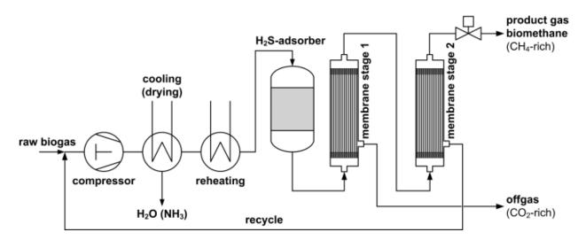
**Figure 5.** Flow sheet of the biogas upgrading plant applying gas permeation in Bruck an der Leitha (Source: Virtual Biogas Project, www.virtuellesbiogas.at)
