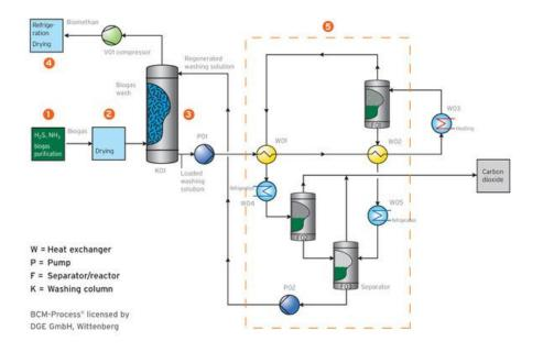
Figure 8. Flowchart of the amine washing process. BCM-Process® licensed by DGE GmbH, Wittenberg (Courtesy: www.mt-biomethan.com)
